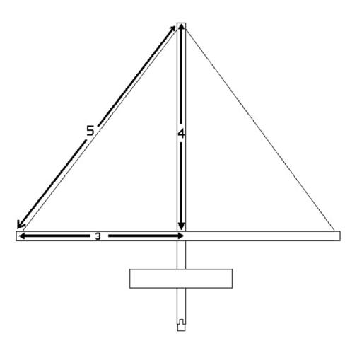
A Pythagorean triangle is a triangle with a right angle, whose sides can be calculated using the Pythagorean theorem:  $a^2 + b^2 = c^2$ . In a 3-4-5 triangle, c = the hypotenuse of the triangle. Try to find materials to make a pump drill that uses the Pythagorean triangle for the best results.
