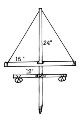
Wooden Pump Drill - The pump drill is a wooden tool that drills little holes/circles into a certain item. Native people have used the pump drill for centuries to start fires and drill holes. This tool was ideal for making holes in bone, wood or shells and for making beads.
